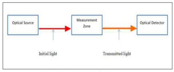
Fig. 2 - Basic working principle of optical sensor
