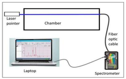
Fig. 4 - Experimental setup for laser stability test
