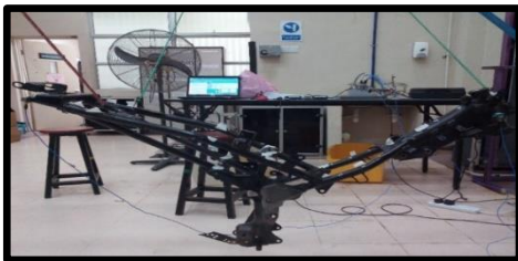
Figure 3. Hanging motorcycle structures under free-free boundary conditions
