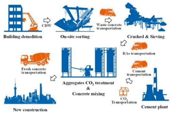
Figure 1: Illustrating the process of concrete production using fully carbonated recycled aggregates (RAs) [20]
