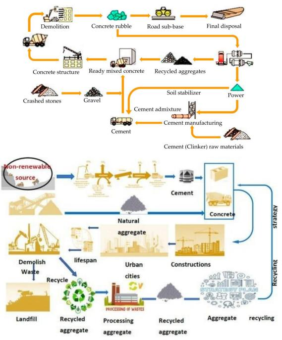
Figure 2: (Top) Production of recycled concrete aggregates (RCAs) from demolished building waste [3]. (Bottom) fundamentals of developing a strategy for recycled concrete aggregates (RCAs) design [31]
