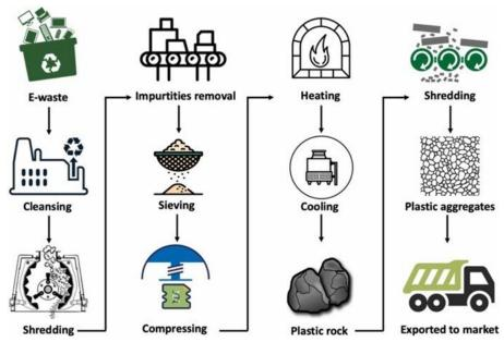
Figure 3: Manufacturing e-waste plastic aggregates through preparation process [25]
