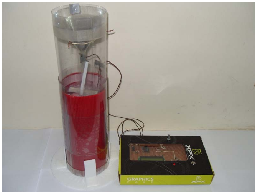
Figure 3.15: The real model of Digital Rain Gauge
