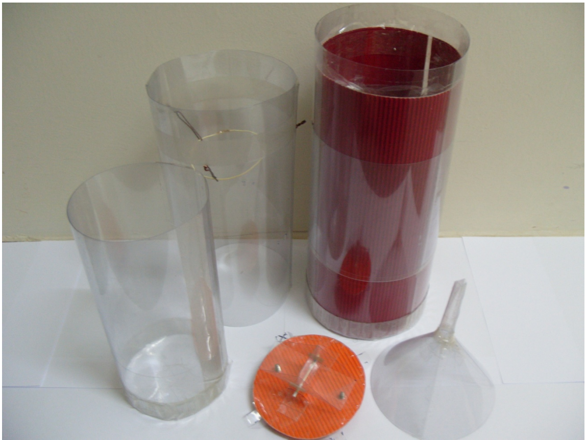
Figure 3.16: The model built consist inner container, outer casing above and below, funnel, and tipping bucket.
