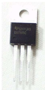
Figure 3.4: Voltage regulator LM7805 and leg descriptions
