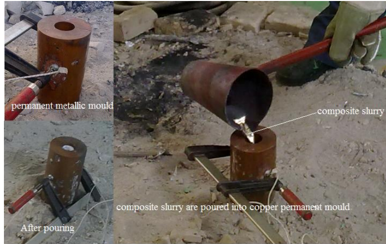
Fig. 1: Pouring the composite slurry into the metallic moulds
