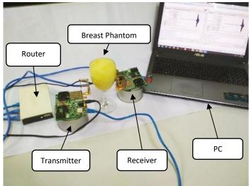
Fig. 4. Experimental setup for breast cancer detection
