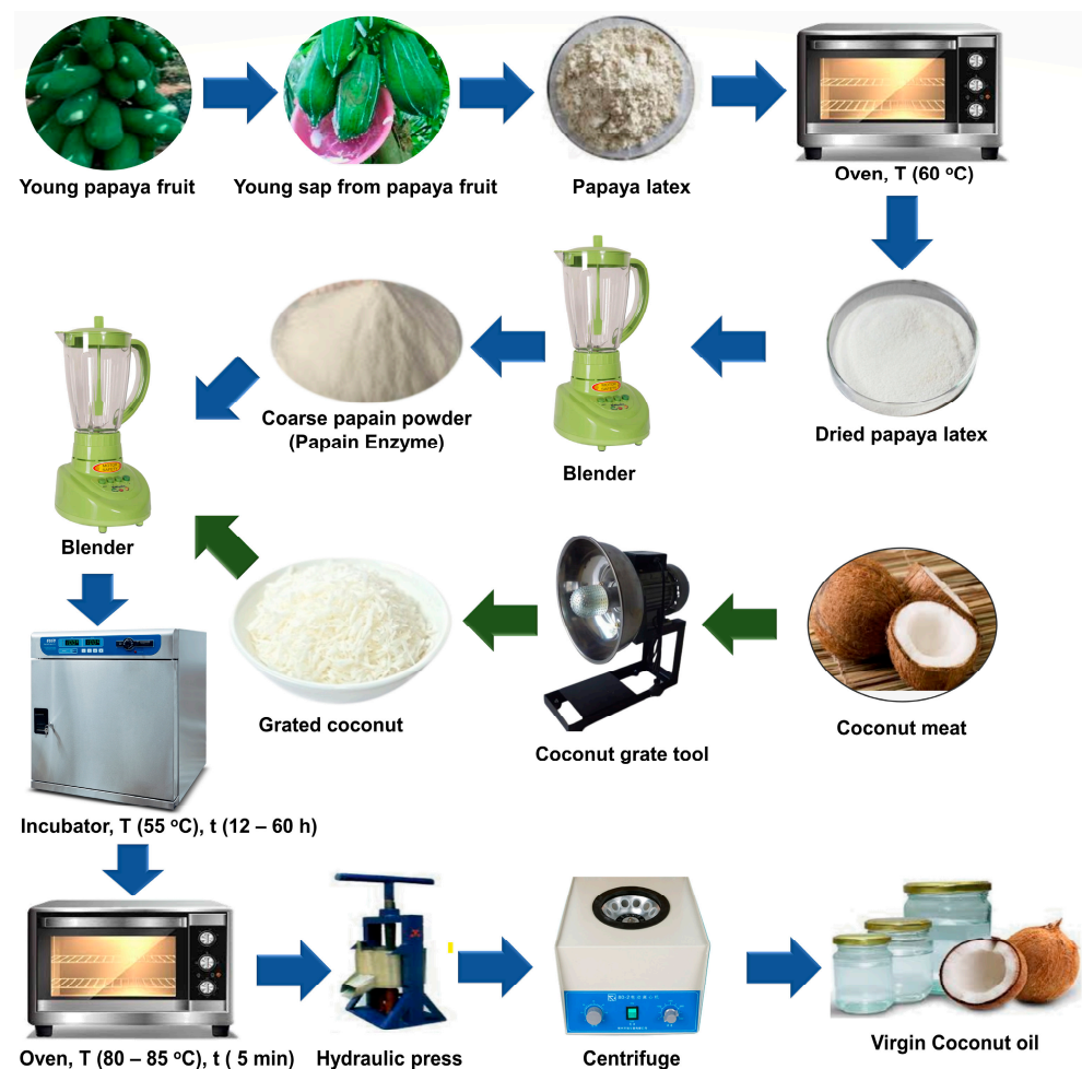
Figure 1. Flowchart of CPE process for VCO production.
