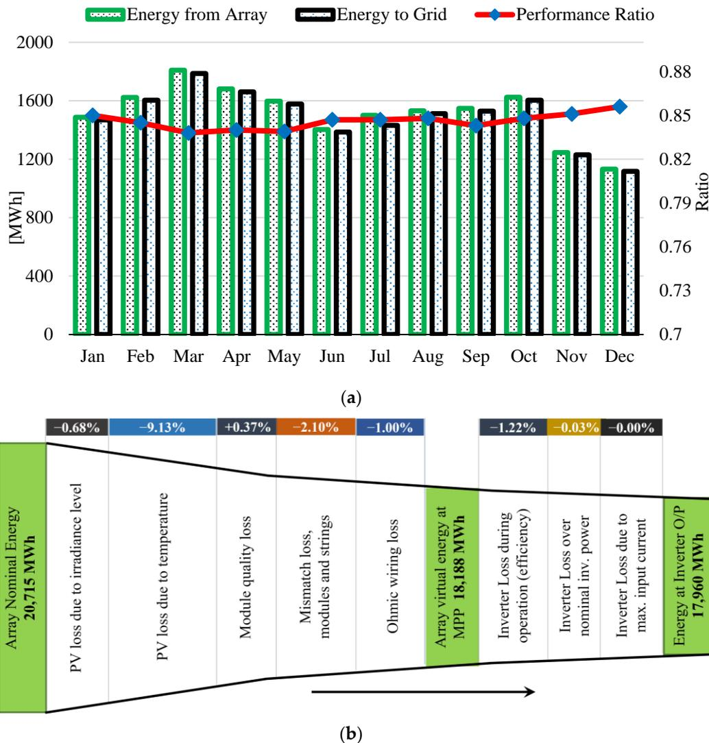
**Figure 9.** (a) Monthly energy production, delivery to grid and performance ratio; (b) Loss diagram of the system.
