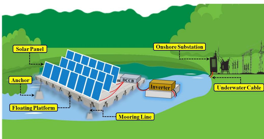
**Figure 3.** Architecture of an FSPV power plant.
