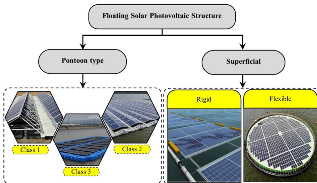
**Figure 4.** Categorization of floating structures of FSPV systems.
