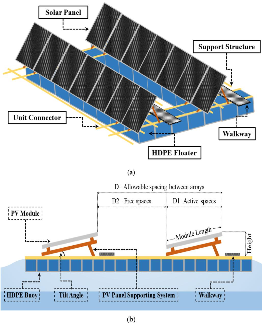
**Figure 8.** (a) Energy generation platform; (b) Unit structure of proposed FSPV.
