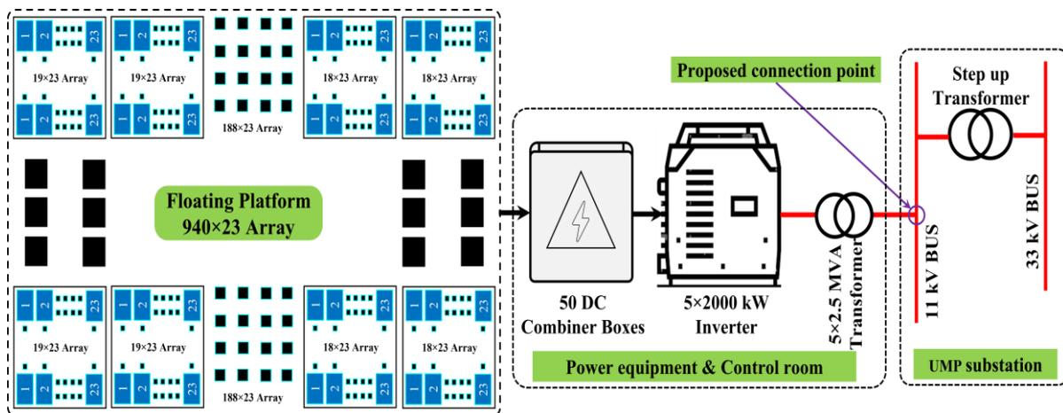
Figure 10. Single line diagram of FSPV plant to TNB grid.
