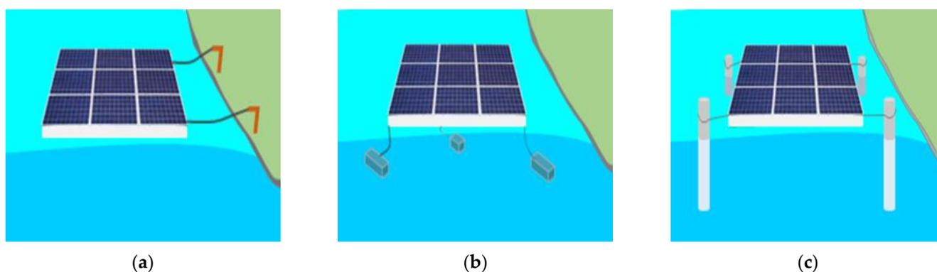
**Figure 5.** Anchoring systems of FSPV plants: (a) bank anchoring; (b) bottom anchoring; (c) piling anchoring.
