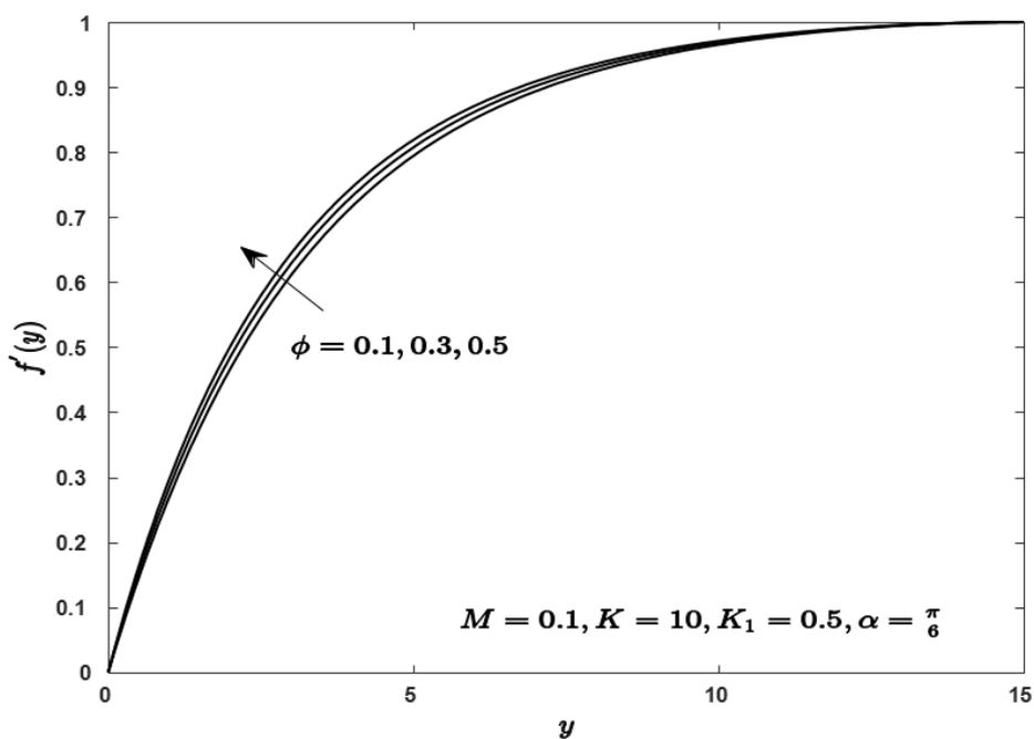
Fig. 3. Velocity distribution for different  $\phi$
