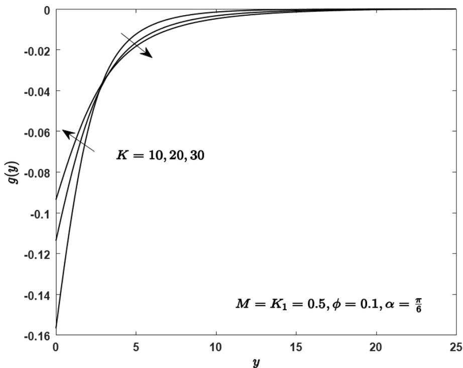
Fig. 7. Microinertia distribution for different  $K$
