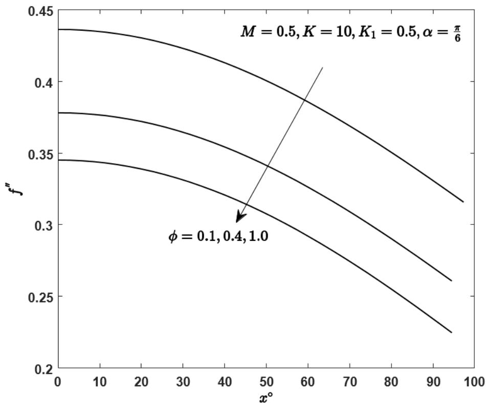
Fig. 2. Variation of skin friction for different  $\phi$
