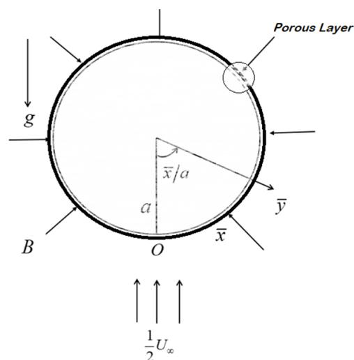
**Fig. 1.** Schematic diagram for the viscoelastic micropolar flow past a porous circular cylinder
