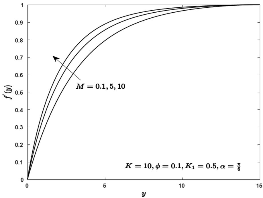
Fig. 9. Velocity distribution for different  $M$
