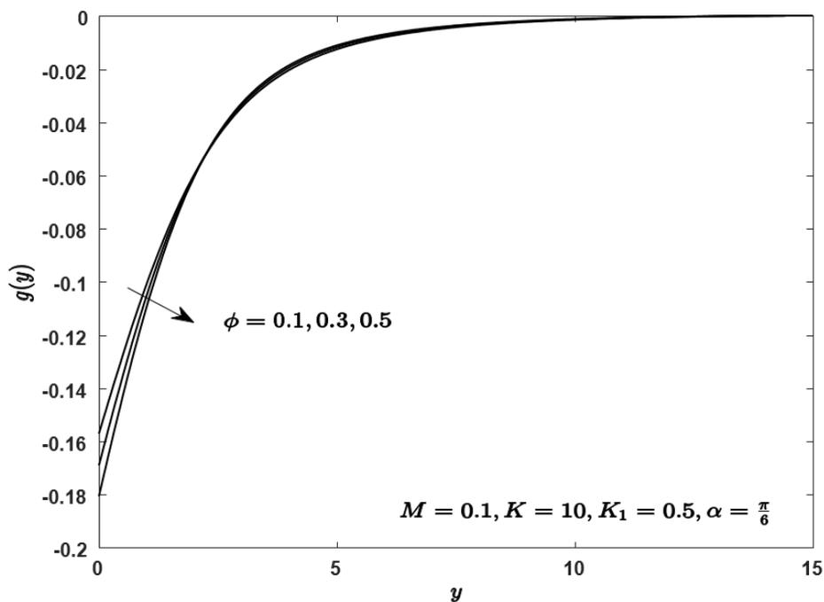
Fig. 4. Microinertia distribution for different  $\phi$
