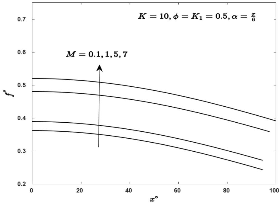
Fig. 8. Variation of skin friction for different  $M$
