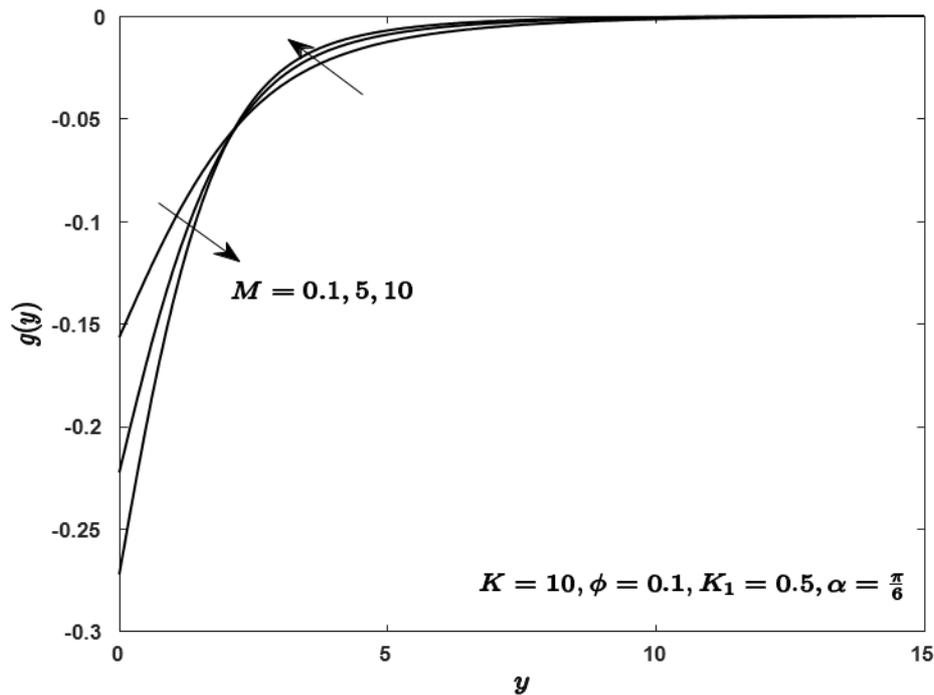
Fig. 10. Microinertia distribution for different  $M$
