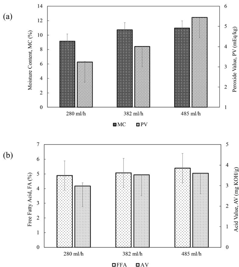
**Fig. 4.** The effect of the feed flow rate of 280, 382, and 485 mL/h on (a) MC and PV and (b) FFA and AV of the microencapsulated *Brevoortia* spp. oil. The MD+GA was used as the emulsion formulation, and the inlet air temperature was 200 °C. Results are expressed as the mean  $\pm$  standard deviation.
