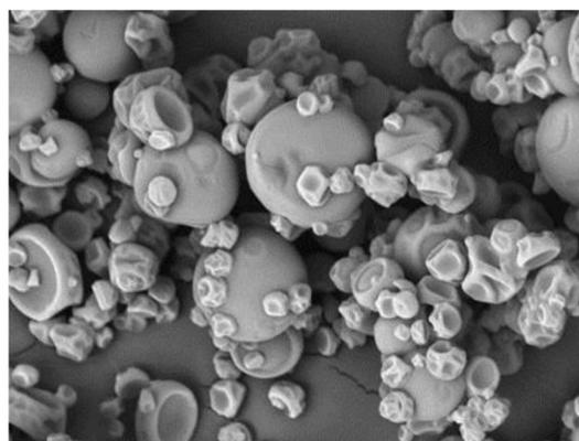
**Fig. 5.** The SEM image of *Monopterus albus* oil extract microcapsules using the MD+GA emulsion formulation produced at an inlet air temperature of 200 °C and feed flow rate of 280 mL/h (2000x magnification).
