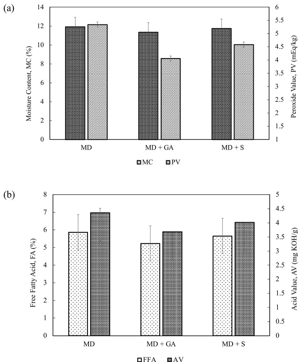
**Fig. 1.** The effect of the MD, MD+GA, and MD+S emulsion formulation on (a) MC and PV and (b) FFA and AV of the microencapsulated *Brevoortia* spp. oil. The inlet temperature, air dry flow, and feed flow rate were set to 190 °C, 2.7 m/s, and 382 mL/h, respectively. Results are expressed as the mean  $\pm$  standard deviation.
