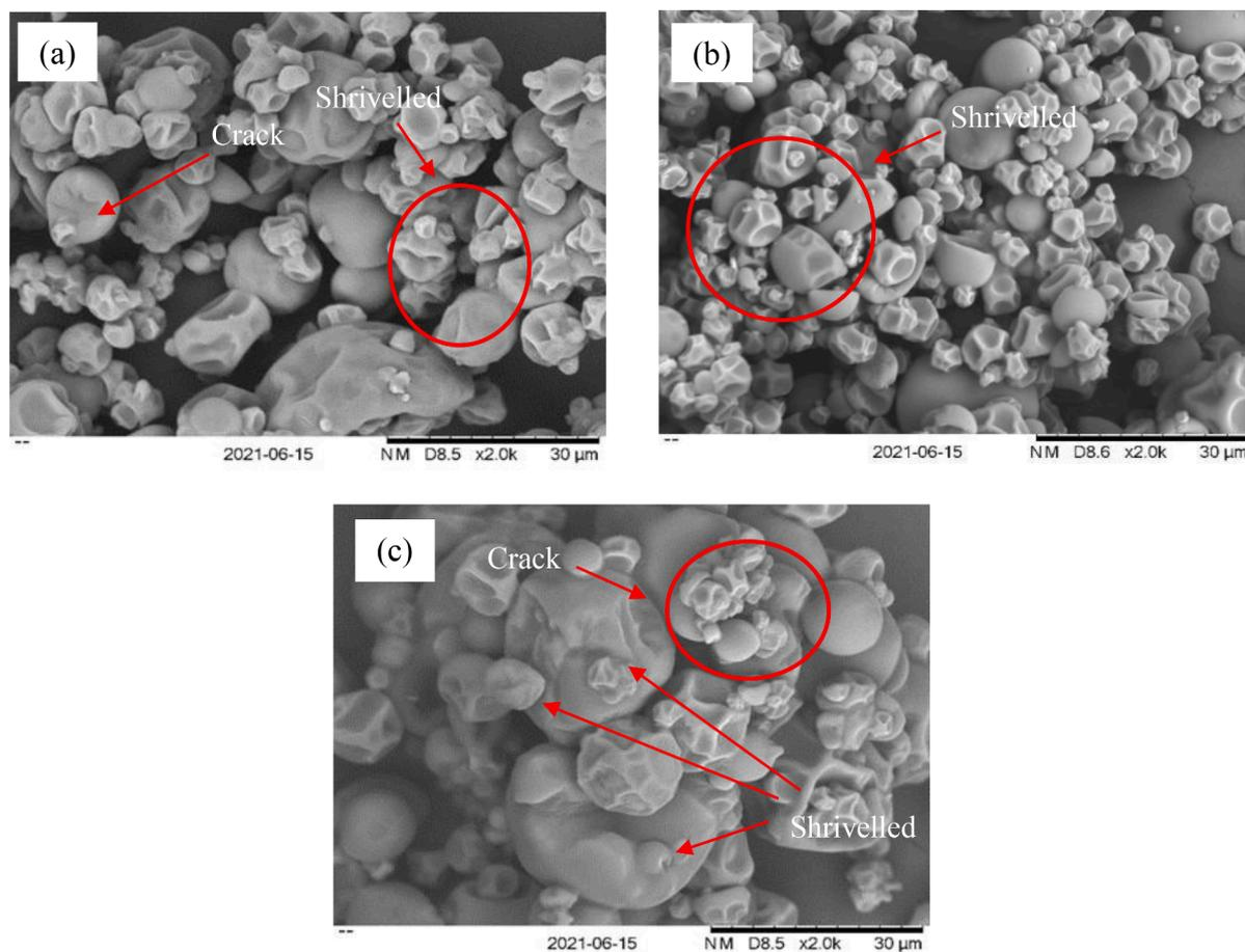
Fig. 2. The SEM images of the microencapsulated *Brevoortia* spp. oil based on (a) MD, (b) MD+GA, and (c) MD+S formulations at 2000x magnification.
