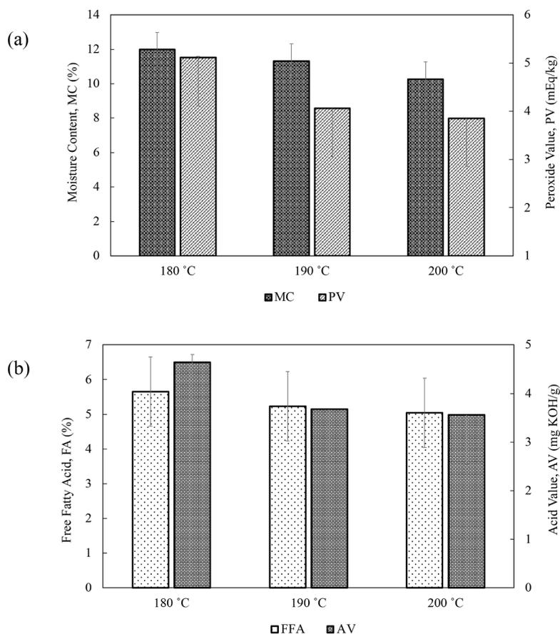
**Fig. 3.** The effect of inlet air temperatures at 180, 190, and 200 °C on (a) MC and PV and (b) FFA and AV of the microencapsulated *Brevoortia* spp. oil. The MD+GA was used as the emulsion formulation, and the feed flow rate was 382 mL/h. Results are expressed as the mean ± standard deviation.
