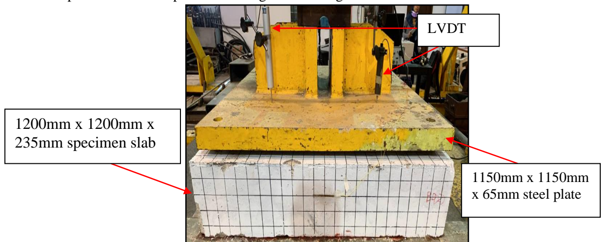
Figure 7. LVDT devices set-up for the slab specimens
