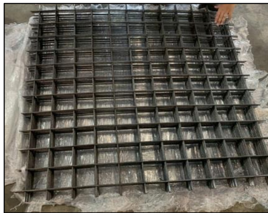
Figure 2. DA6 BRC reinforcement.
