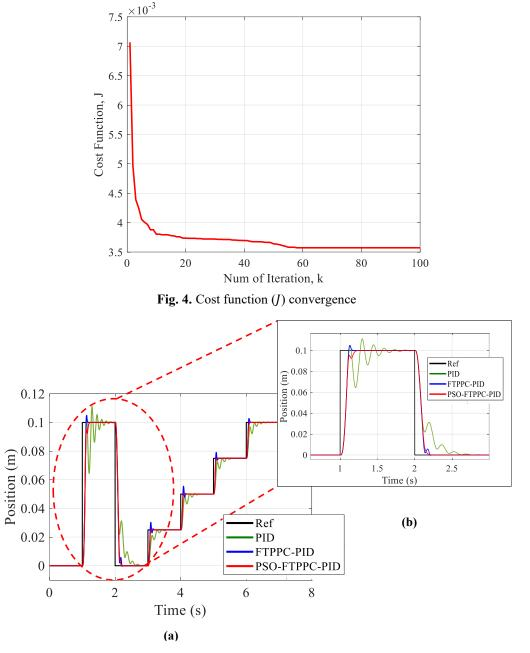
Fig. 5. Sample of multi-step displacement responses on PPDVC rod-piston position performances; comparison between PSO-FTPPC-PID, FTPPC-PID, and PID; (a) Overall time sample (b) Zoom-in view sample
