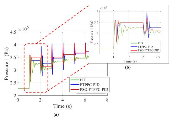
Fig. 7. Sample of pressure in Pressure 1 performances between PSO-FTPPC-PID, FTPPC-PID, and PID on PVDC; (a) Overall time sample (b) Zoom-in view sample
