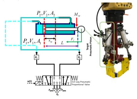
Fig. 1. PPVDC hardware schematic with TPG [14]
