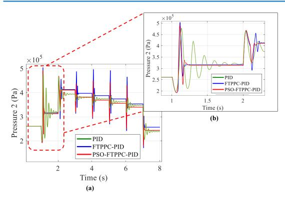
Fig. 8. Sample of pressure in Pressure 2 performances between PSO-FTPPC-PID, FTPPC-PID, and PID on PVDC; (a) Overall time sample (b) Zoom-in view sample
