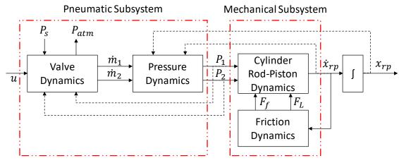
Fig. 2. Mathematical model of the PPVDC structure [14]
