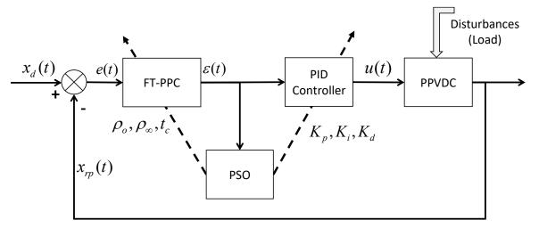
Fig. 3. FT-PPC and PID with PSO control architecture overview for PPVDC rod-piston positioning
