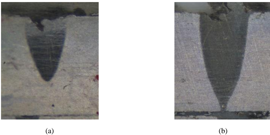
Figure 3. Cross-sectional analyses of the welded joint based on distinct parameter group, (a) Half Penetration from G1 and (b) Full Penetration from G2.
