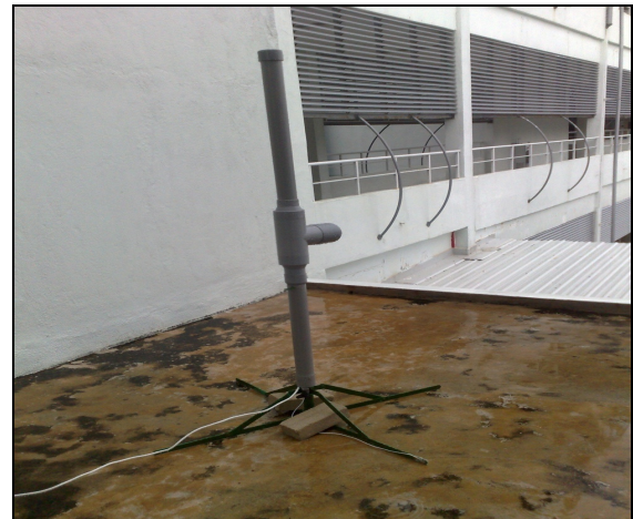
Figure 2. Wire Antenna to detect EF signals
