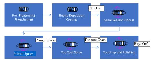
Figure 3. Detail Process for Automotive Paint
