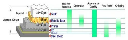
Figure 4. Layers of coating and its properties [10]
