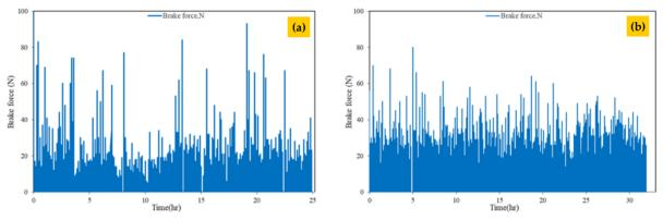
Figure 7. Brake pedal force applied during hilly road (a) and flat road (b)
