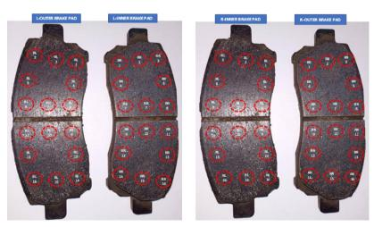
Figure 3. Brake pad measurement point selection
