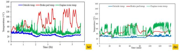
Figure 6. Brake pad temperature generated during hilly road (a) and flat road (b)
