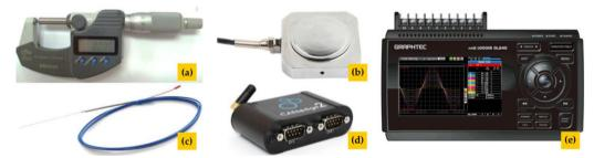
**Figure 1.** Measuring instruments: (a) Micrometer (0-25mm range); (b) Brake pedal force sensor; (c) K-type thermocouple; (d) CANedge2 logger; (e) Graphtec data logger
