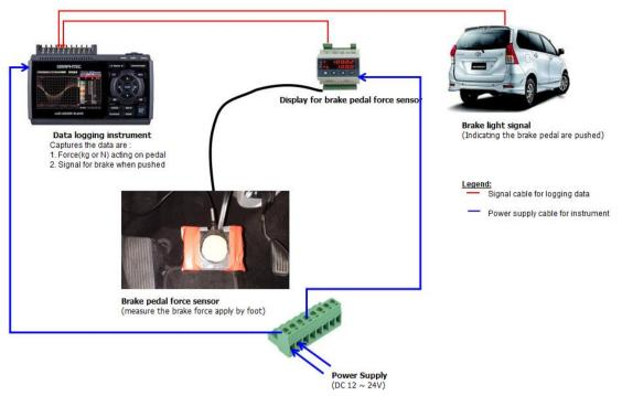
Figure 4. Brake pedal force sensor system setup on the experimental vehicle
