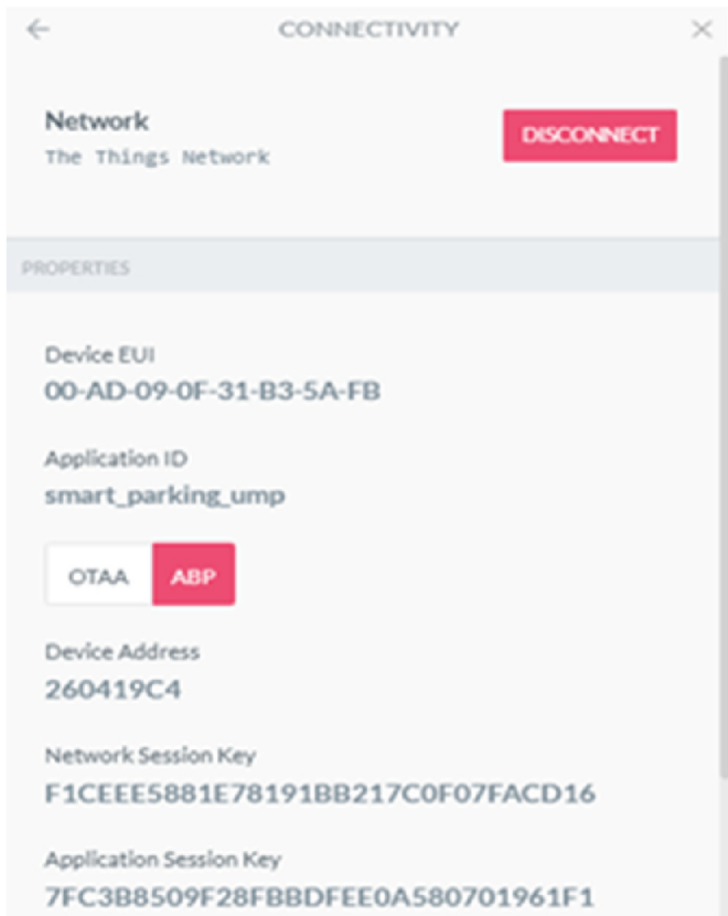
Fig. 10. Successfully received data at the TTN platform.
