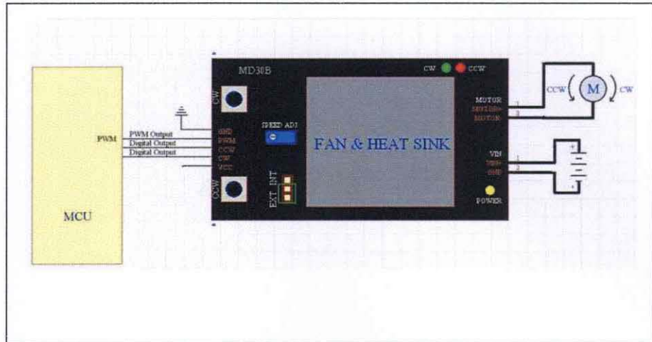
Figure 3.6: MD30B combining with microcontroller
