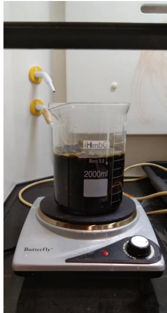
Figure 3.2 Boiling process of pineapple leaf with distilled water and NaOH at constant temperature of 100-degree Celsius.
