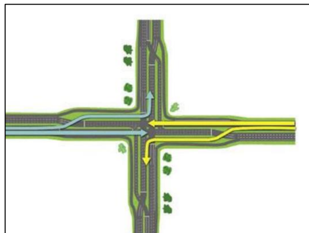
Figure 2.8 Continuous Flow Intersection (Lee, 2013).
