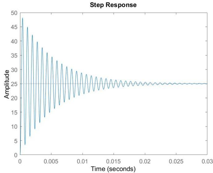
**Figure 4.5 Output response of uncontrolled DC-DC Boost converter**
