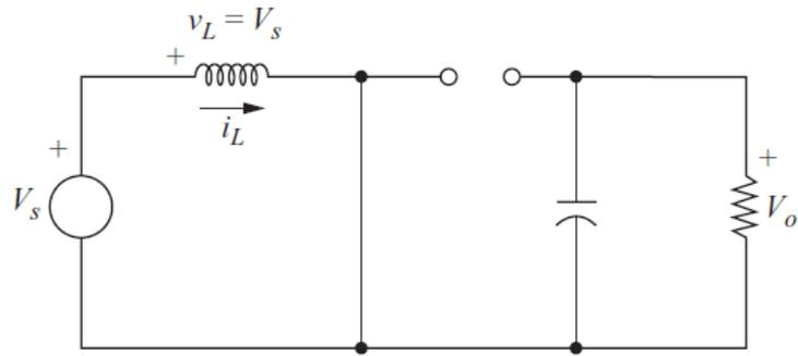
**Figure 3.6 Circuit when the switch closed**
