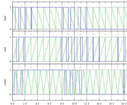
**Figure 2.1 The PWM waveforms using the intersection method**
