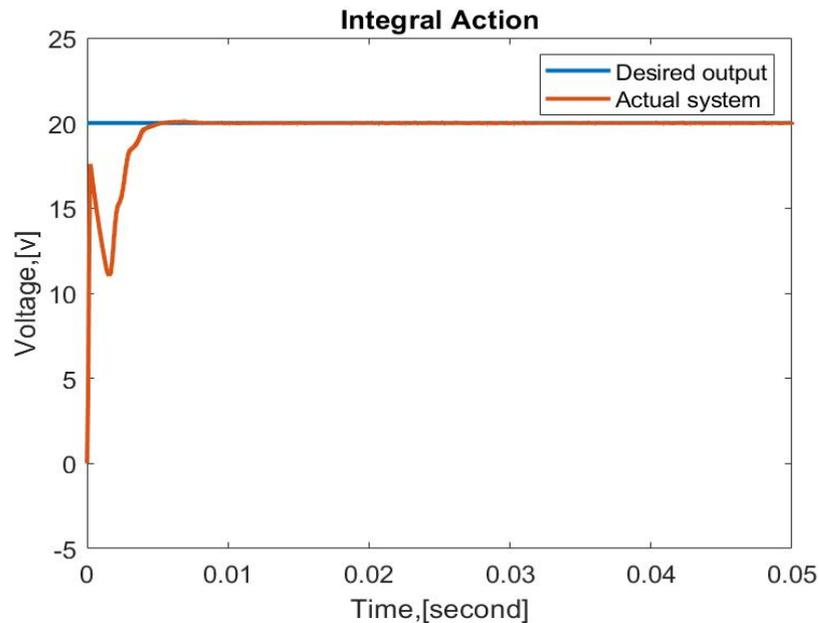
**Figure 4.7 Output response of State-Feedback with Integral action**
