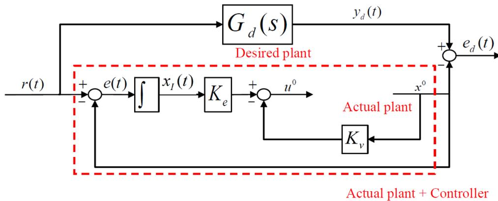
**Figure 3.3 Block diagram of the Fictitious Reference Interactive Tuning**
