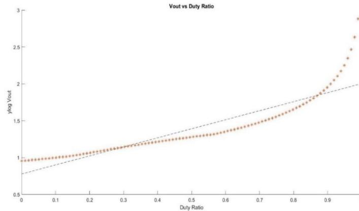
**Figure 4.2 The relationship between the output voltage and duty ratio by using LSM**
