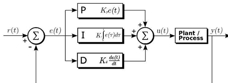
**Figure 2.3** The block diagram of a PID controller in a feedback loop
