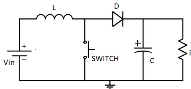
**Figure 1.1 Basic schematic diagram of a DC-DC Boost converter**
