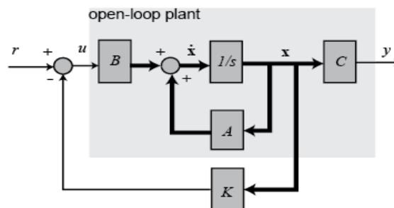
**Figure 3.11 Full State Feedback block diagram**
