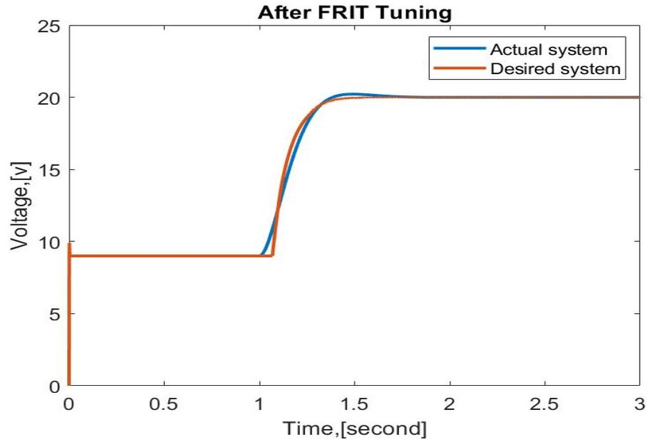
**Figure 4.9 Output response after FRIT tuning**
