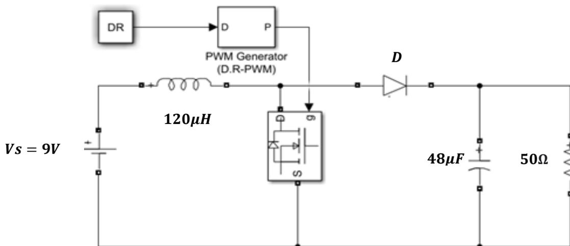
**Figure 3.9 DC boost design in MATLAB Simulink**
