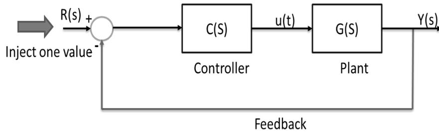
**Figure 1.2 Block diagram of a closed-loop system**
