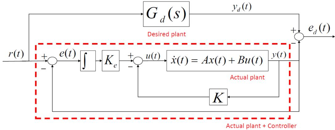
**Figure 3.2 State Feedback with Integral action**
