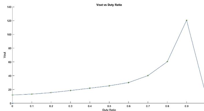
**Figure 4.1** The relationship between the duty ratio and the output voltage of the DC-DC Boost converter
