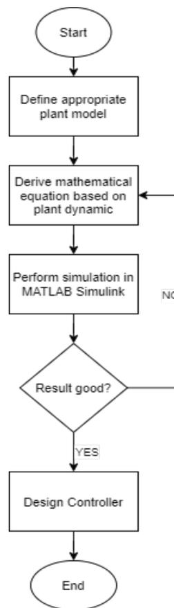
**Figure 3.4 Plant model's flow chart**
