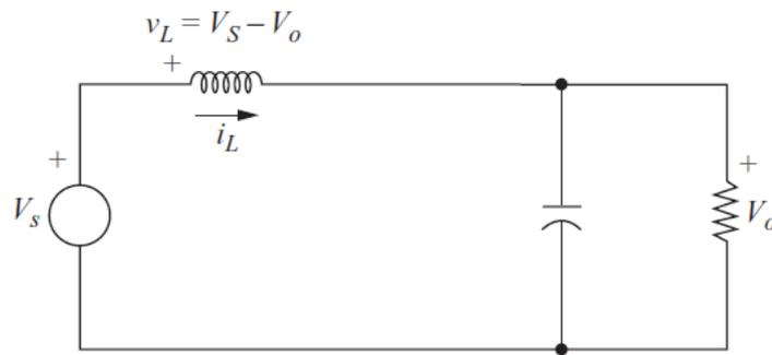
**Figure 3.7 Circuit when the switch opened**
