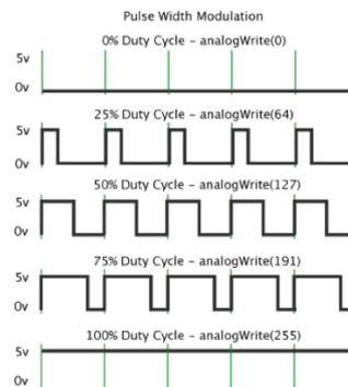
**Figure 2.2 Pulse Width Modulation waveform controlled by Arduino**
