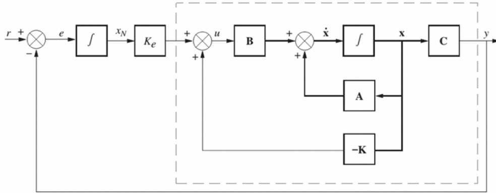
**Figure 3.12** The structure of State-Feedback with Integral action
