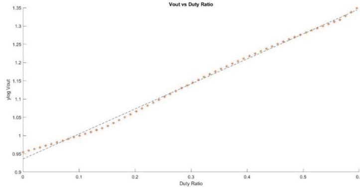
**Figure 4.3 The relationship between the duty ratio and the output voltage using LSM in 60 data points**
