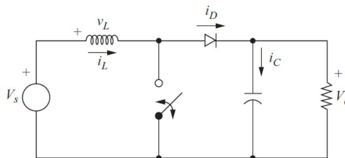
**Figure 3.5 Standard boost converter circuit**
