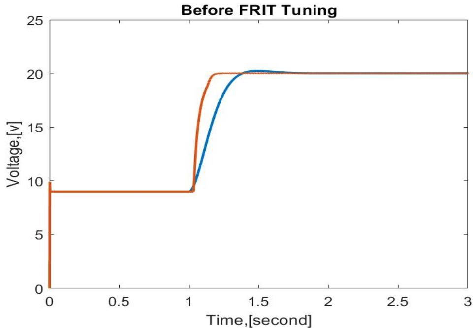
**Figure 4.8** Output response before FRIT tuning
