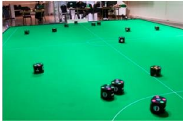
Figure 1.1 The soccer robots of NEUIslanders group that utilize the fuzzy controller in a football game of RoboCup competition. The obtained experimental comes about fulfill the application of fuzzy controllers in control of omnidirectional robots[5].
