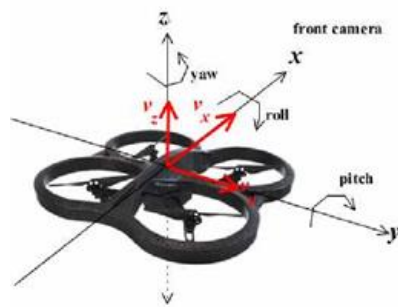
Figure 1.2 Fuzzy Logic Controller (FLC) is actualized within the AR.Drone quadrotor in arrange to form it take after a given trajectory reference. The distance between the position and angle of the AR.Drone to the reference point is utilized as the input of FLC[6].
