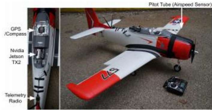
Figure 2.2 The Carbon-Z T-28 fixed-wing UAV platform equipped with an on board computer and additional modules for our dataset collection [1]
