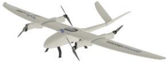
Figure 2.5 German drones Songbird VTOL UAV [9]
