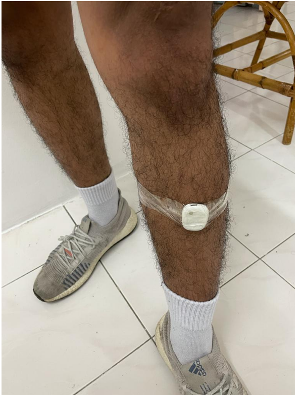
Figure 3.3.9: IMU Sensor on left shank of subject
