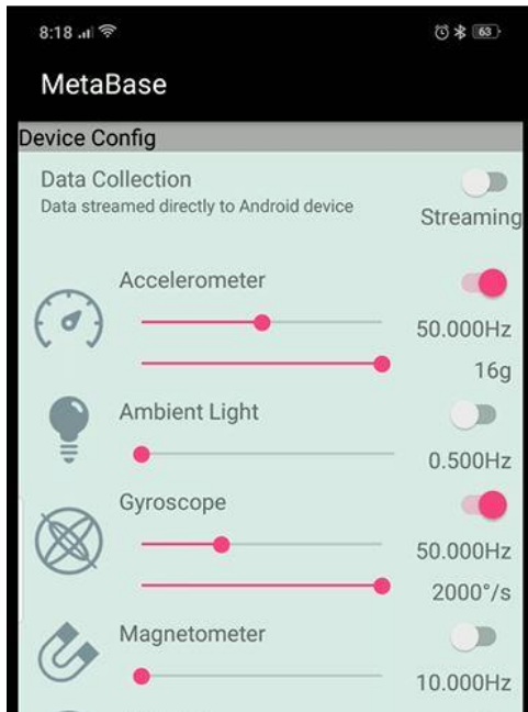
Figure 3.3.3.11 Metabase Accelerometer and Gyroscope Parameter Settings
