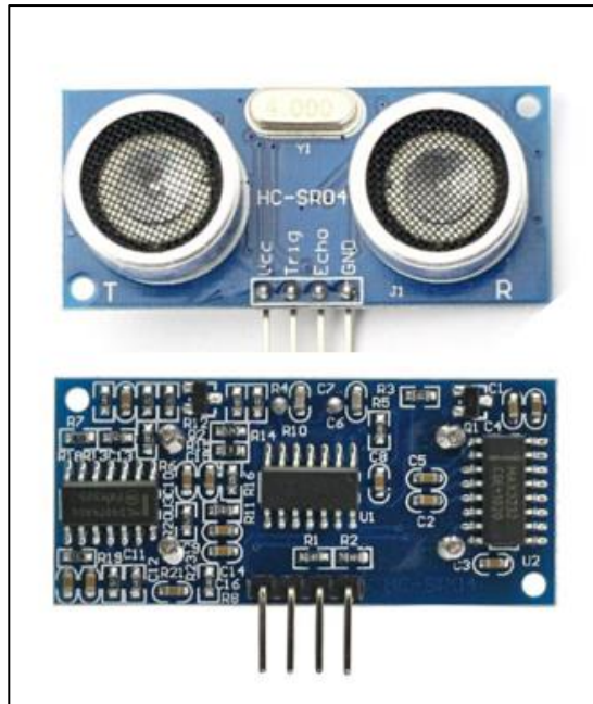
Figure 3.6 HC-SR04 Ultrasonic Sensor ( Complete Guide for Ultrasonic Sensor HC-SR04 with Arduino / Random Nerd Tutorials, n.d. )
