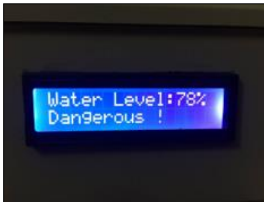
Figure 4.5 The LCD Display shows the Danger Situation
