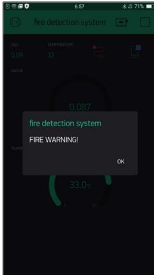
Figure 4.8 Blynk notification when sensor detected heat over threshold limit
