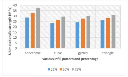
Figure 2: Average ultimate tensile strength of the various infill pattern and infill percentage
