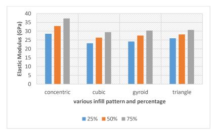
Figure 3: Average elastic modulus of the various infill pattern and infill percentage
