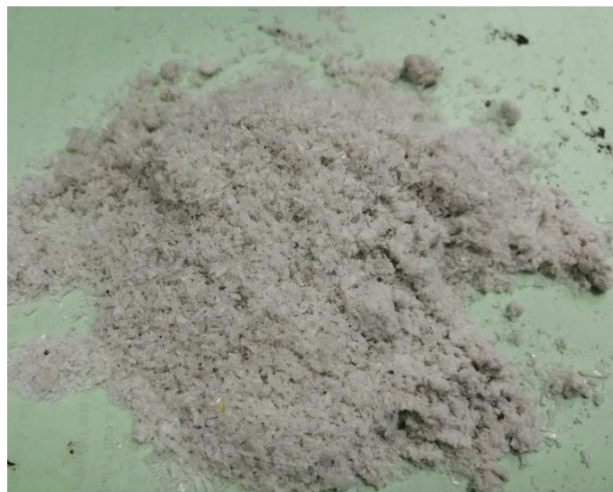
Figure 2. Plastic size 0.425 to 0.075mm used to coat the aggregate.
