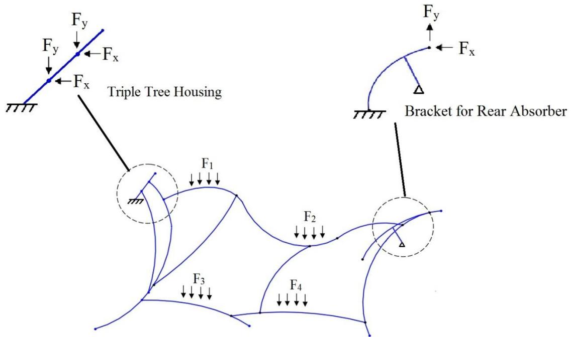
Figure 6. Loads transfer to triple tree housing and bracket absorber rear.
