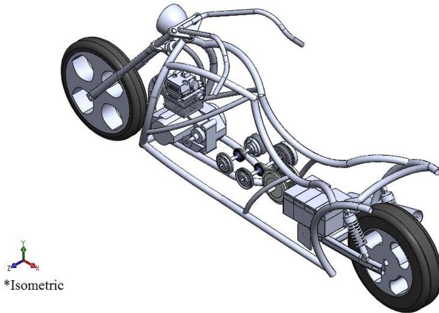
Figure 3. Chassis 3D modeling intergraded with PHEM components and drive-train mechanism.
