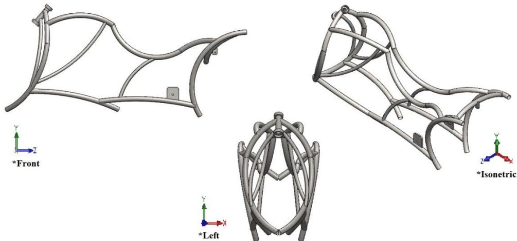
Figure 2. Chassis 3D modelling with CAD software SolidWorks 2012.
