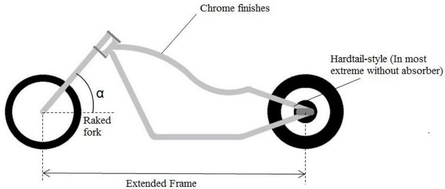
Figure 1. Features in Chopper type motorcycle.
