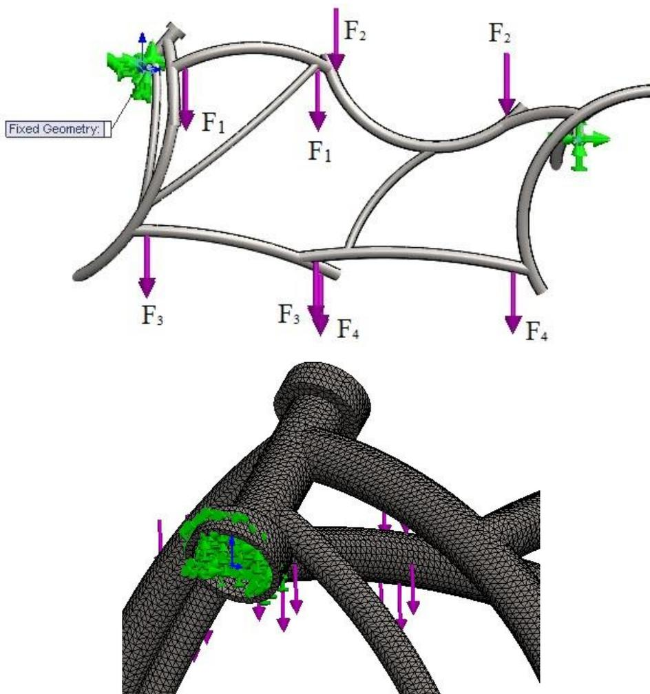
Figure 5. Chassis 3D model with fixtures, loads and meshing.
