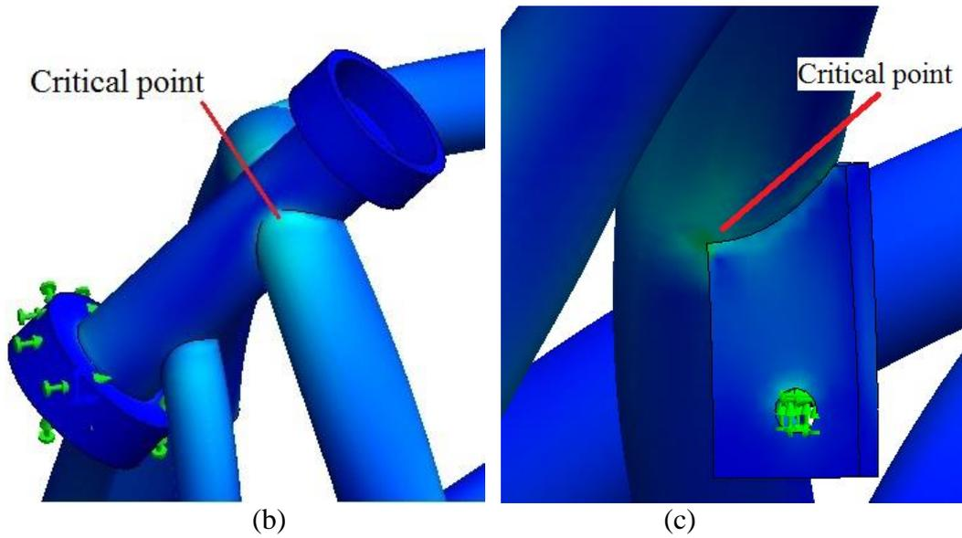
Figure 7. Simulation result (von Mises Stress).
