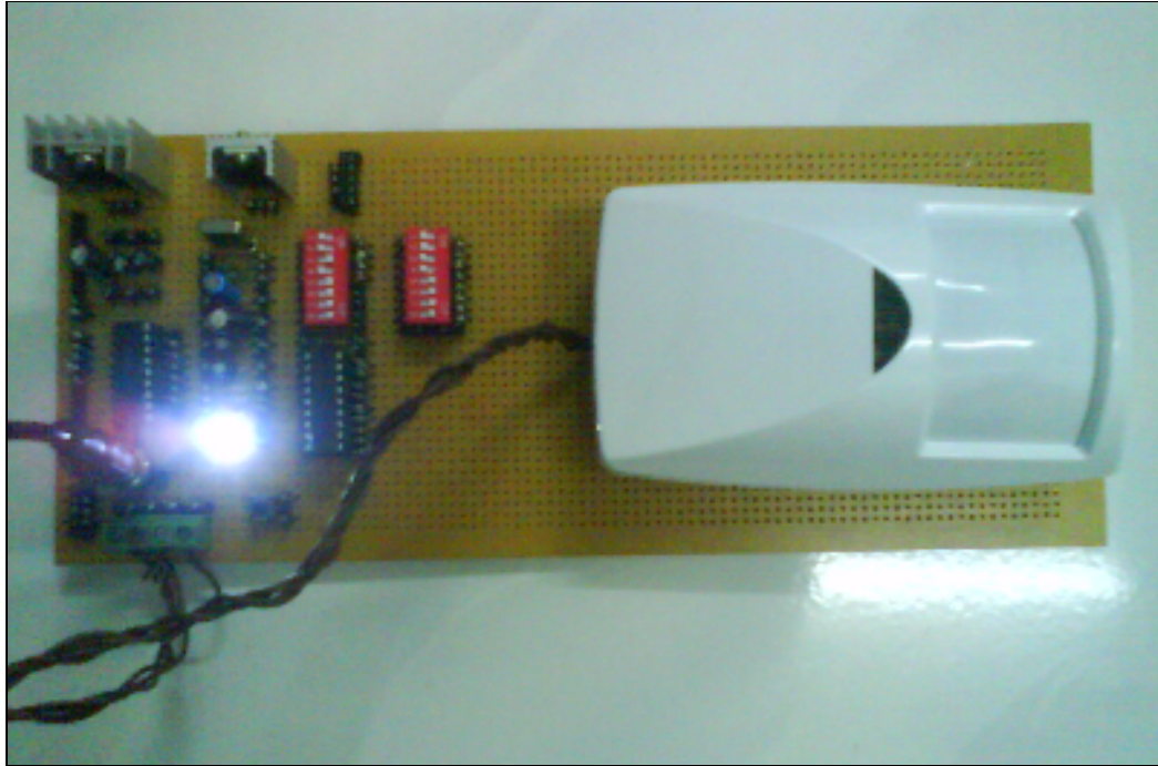
Figure 4.4 Motion detected by PIR sensor and LED is ON
