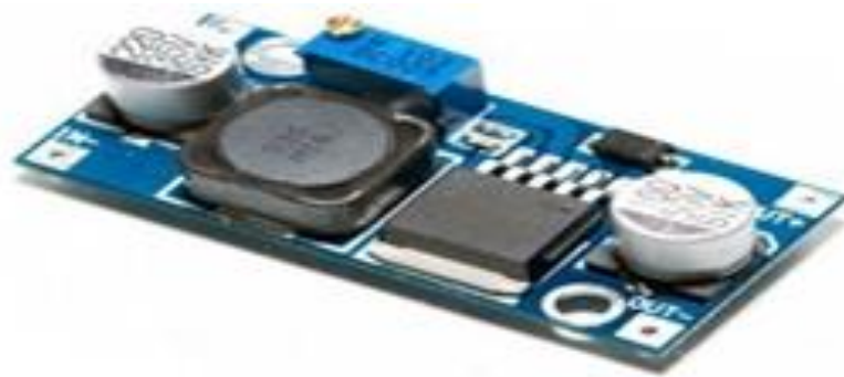
Figure 2.12 DC boost converter
