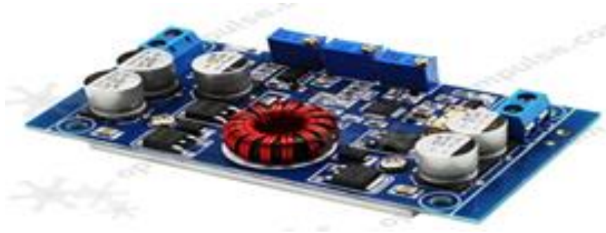
Figure 2.11 Buck boost converter
