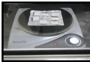
Figure 3. 74: Baked FTO glass 450^\circ\text{C} for 45 minutes for Second Batch
