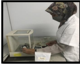
Figure 3. 54: Weighing \text{TiO}_2 powder by using Analytical Balance for First Batch
