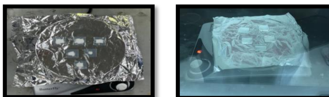
Figure 3. 62: Baked FTO glass 450^\circ\text{C} for 45 minutes for first batch
