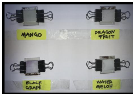
Figure 3. 80: Assembly the Photoelectrode & Counter Electrode for Second Batch
