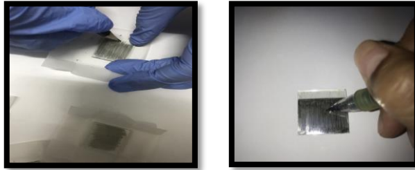
Figure 3. 79: Shaded Counter Electrode for Second Batch with graphite
