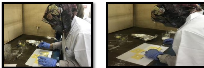
Figure 3. 60: A drop of \text{TiO}_2 on the FTO glass and using Doctor Blade Method
