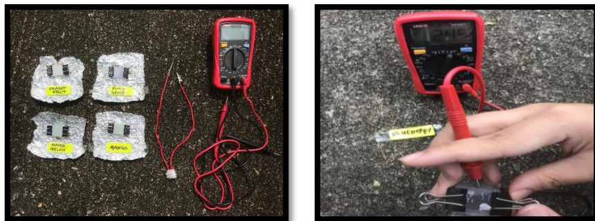
Figure 3. 86: Measurement of Voc under direct sunlight
