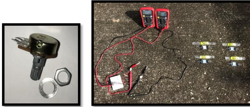
Figure 3.88: Measurement of voltage at load
