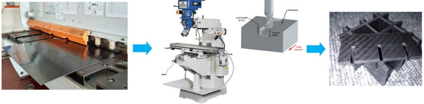
Fig. 4. Fabrication procedure of SRPP sheet for SRPP honeycomb sandwich panel.
