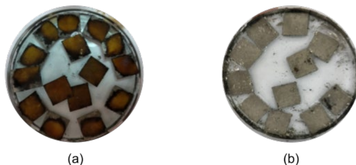
Figure 1: Physical appearance of (a) NiNPs/FP and (b) NiNPs/CS-FP
