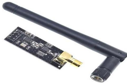
Figure 3. 14 RF NRF24L01+ transceiver module[40]
