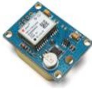
Figure 3. 12 GPS NEO-7M Module[38]
