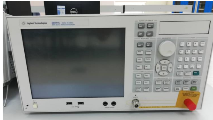
Figure 18: Agilent Vector Network Analyzer (VNA)
