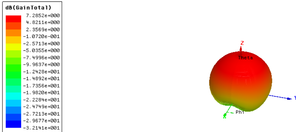
Figure 4.10 3D polar plot gain Teflon with SIW addition
