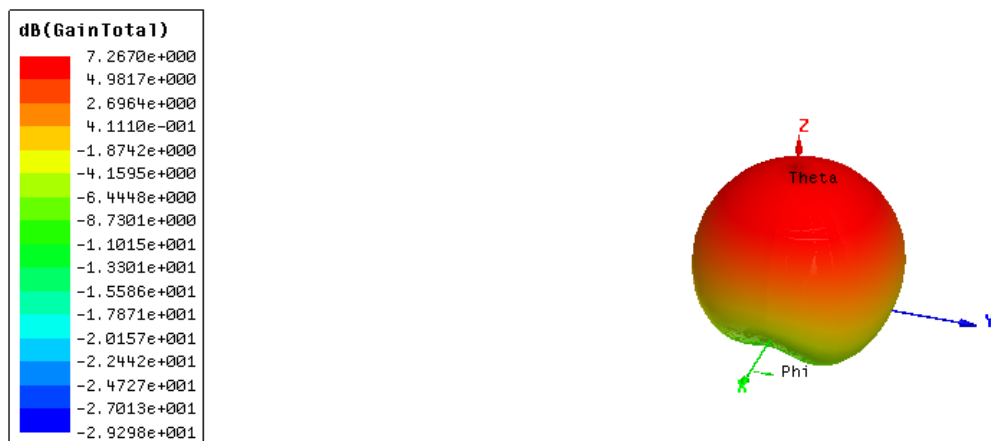
Figure 4.9 3D polar plot gain of Teflon
