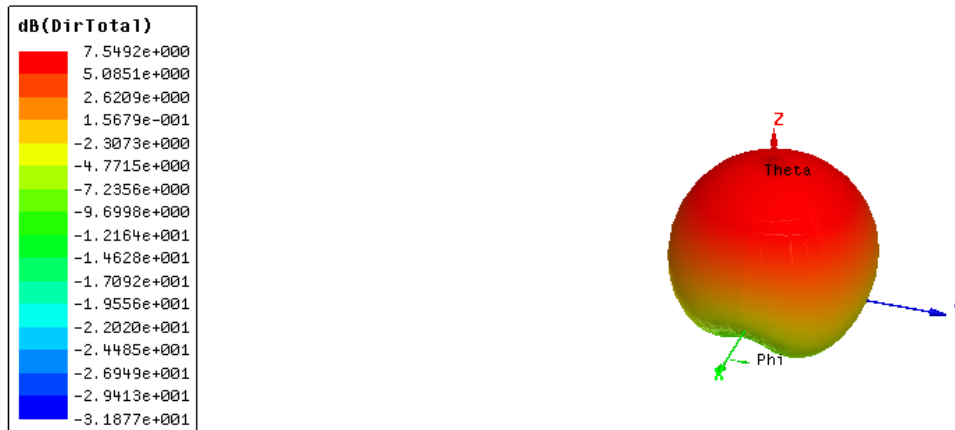
Figure 4.12 Directivity of the Teflon with SIW addition
