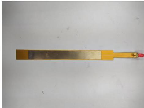
Figure 3.5 Front side of the sensor and sensing area
