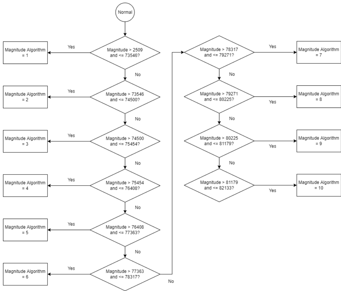
Figure 3.6 Flowchart of magnitude algorithm conversion for normal dataset
