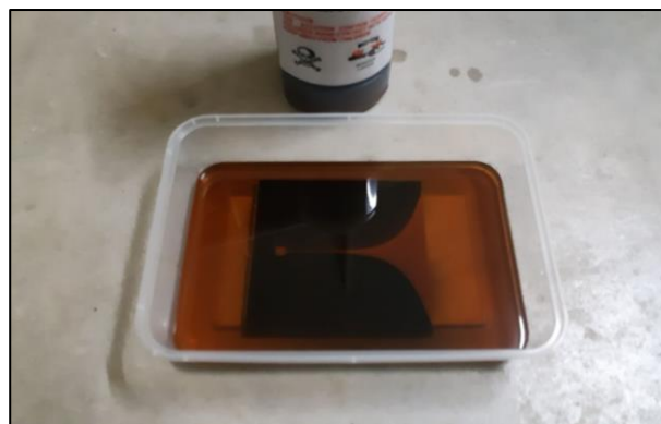
Figure 3.19 PCB Submerge into the Etching Chemical.
