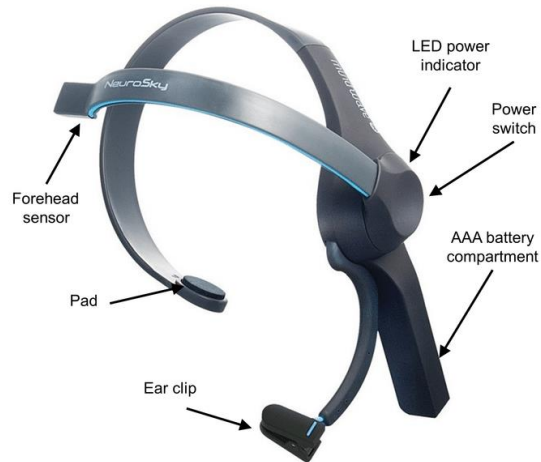
Figure 3.7 NeuroSky Mindwave Mobile Headset with labeling parts.
