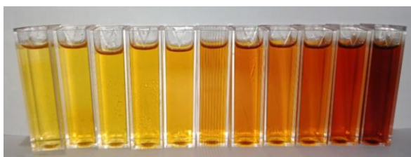
Figure 16: 10 palm oil samples were heated repeatedly.
