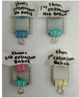
Figure 4. 10: The different completeness TiO 2 between non pre-heated and pre-heated
