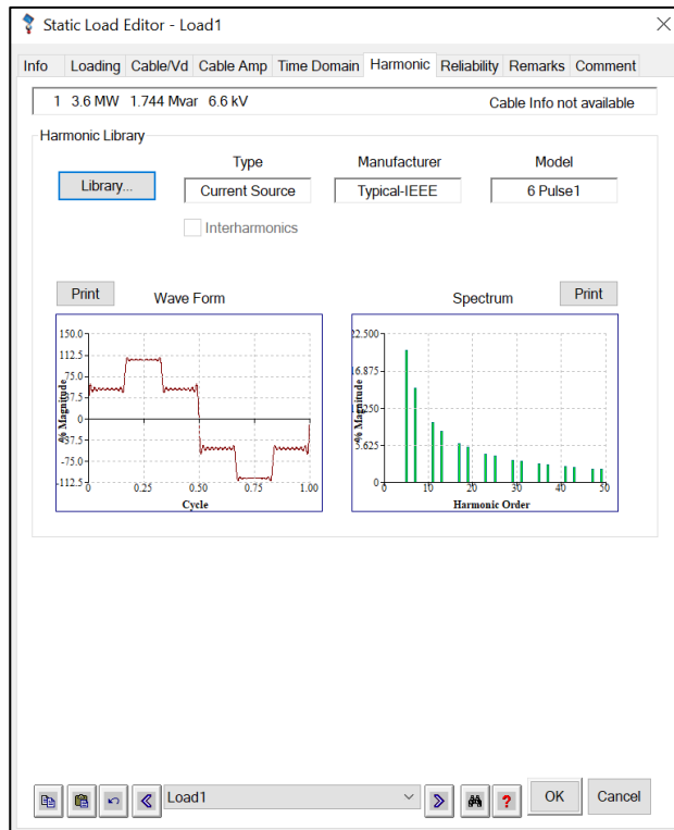
Figure 3.9 Harmonic type, waveform and spectrum
