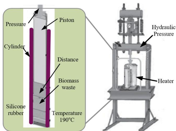
Fig. 2. Schematic diagram to process biocoal.
