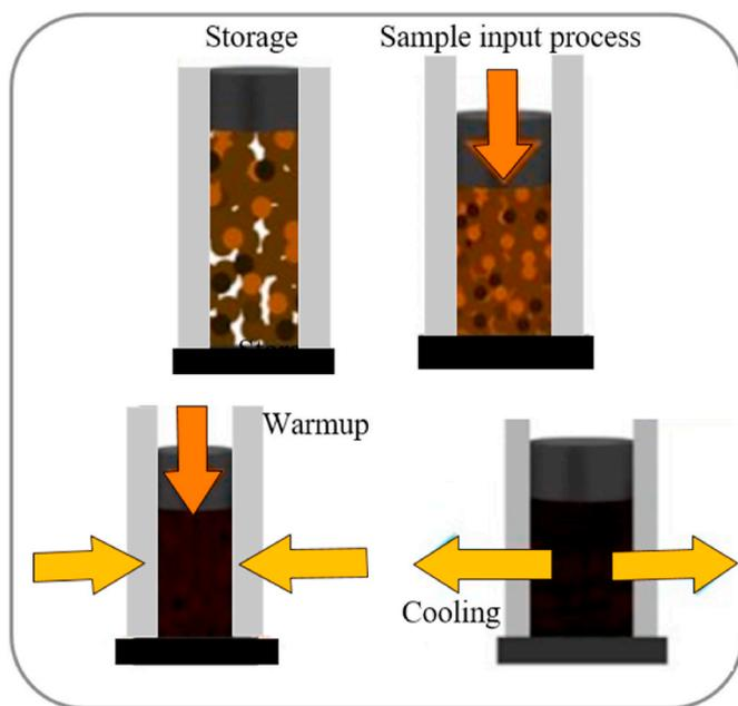
Fig. 3. Procedure of production biocoal.
