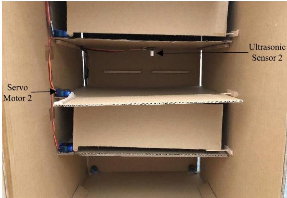
Figure 2.2.1.6 Position of Sensors Side View for Each Compartment.
