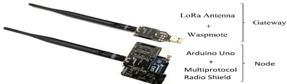
Figure 2.2.1.4 LoRa Gateway Equipment.
