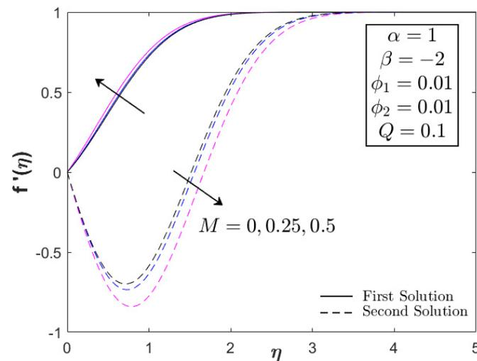
**Figure 10.** Velocity profile of  $\text{Fe}_3\text{O}_4\text{-CoFe}_2\text{O}_4/\text{H}_2\text{O}$  with different  $M$ .
