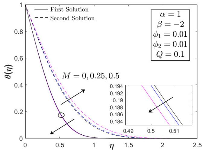
Figure 11. Temperature profile of  $\text{Fe}_3\text{O}_4\text{-CoFe}_2\text{O}_4/\text{H}_2\text{O}$  with different  $M$ .
