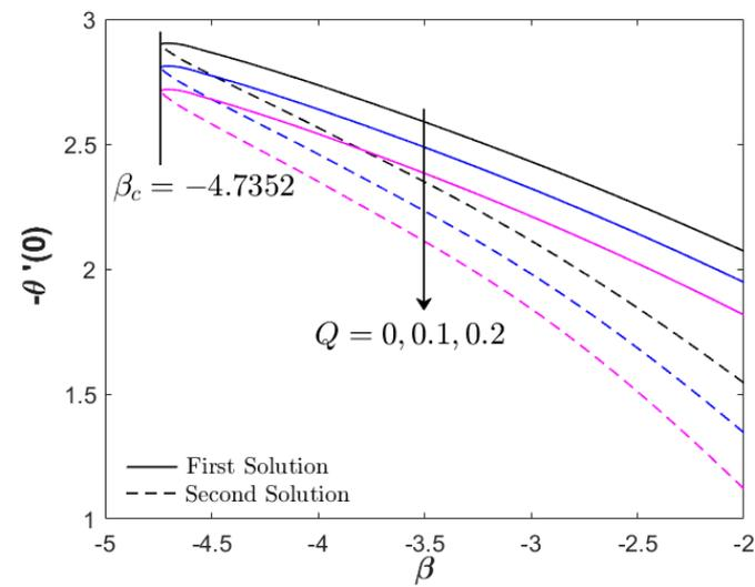
Figure 4.  $-\theta'(0)$  for various  $Q$  (heat generation parameter).
