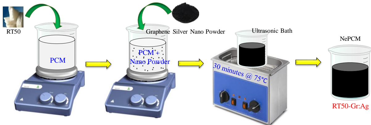
Figure 1. Preparation of RT50-Gr:Ag composite PCM using bath ultrasonicator.
