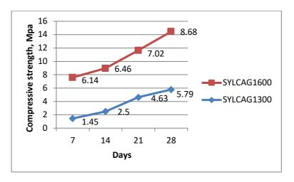
Fig. 1. Compressive strength of SYLCAG
