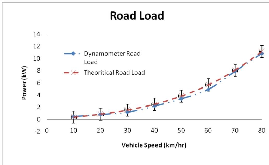
Figure 16: Road load data comparison between data from roll down test and engine dynamometer
