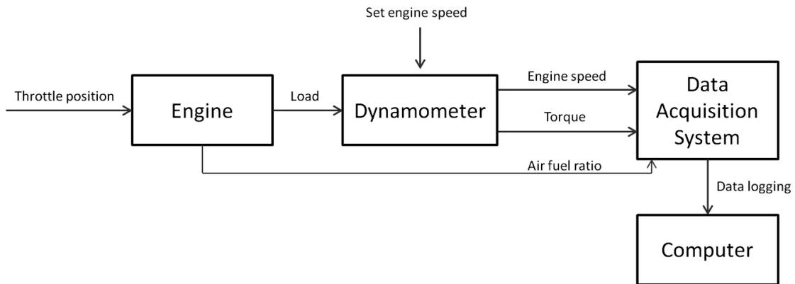
Figure 6: Engine dynamometer schematic
