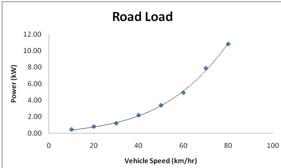
Figure 15 : Road load power from engine dynamometer data
