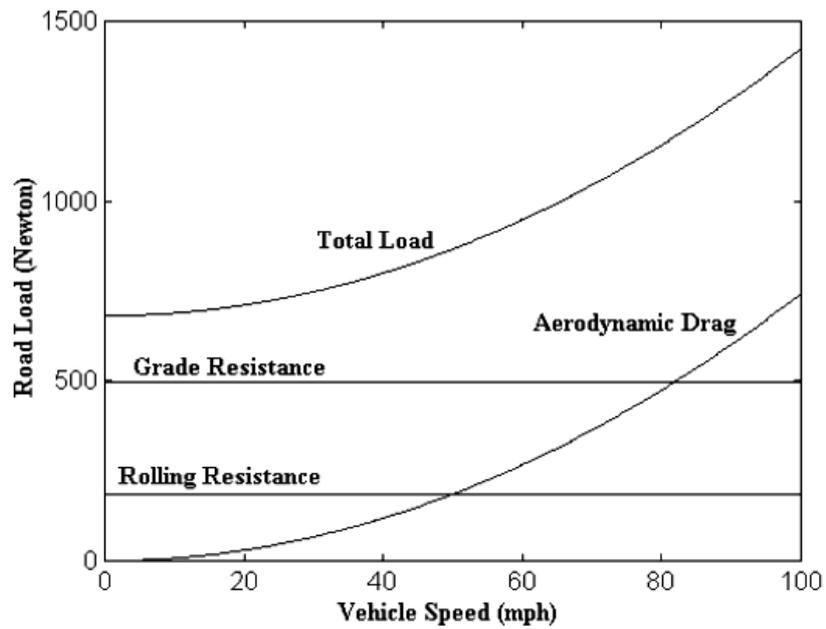
Figure 1: Typical Vehicle Load Function
