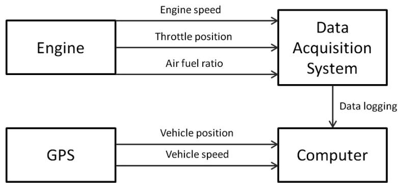
Figure 5: Vehicle instrumentation schematic
