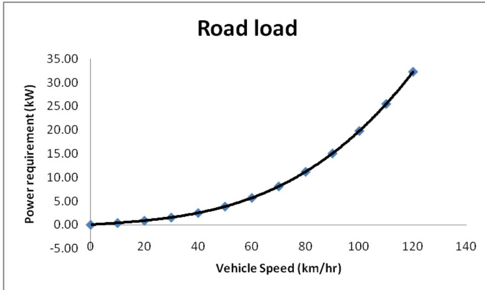
Figure 14: Simulated road load using average data from roll down test
